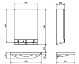
As a tailor-made washbasin solution for row installation From our Varius range, choose the ETON trough with a back wall. The washbasins are made of Miranit, a synthetic resin-bonded mineral material.
